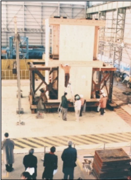
Canadian and Japanese engineers performing a shake table test of a two-storey shear wall at Japan's National Research Institute for Earth Science and Disaster Prevention.
