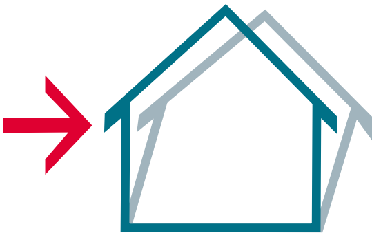
A lateral force is a sideways motion that can make a building rack (as shown), overturn or slip off its foundation.
